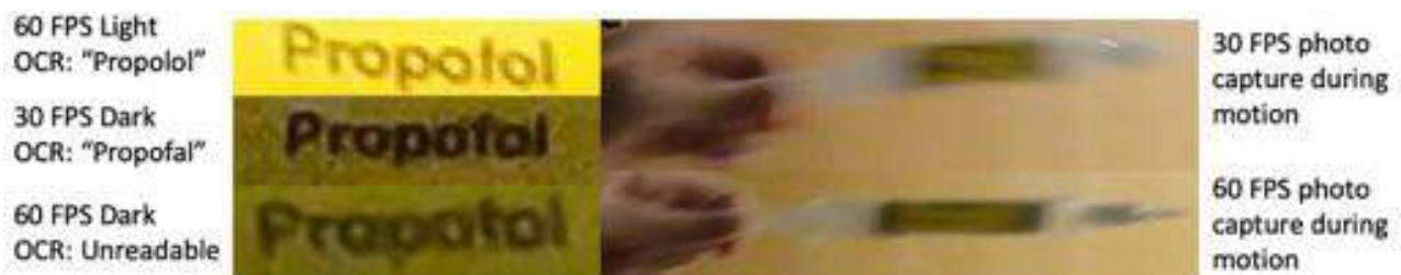
Figure 4: In dark rooms, lower frames per second (FPS) performs better at optical character recognition (OCR) in static conditions (left), but has more blur with movement (right)
